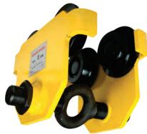
Rolacrawl hoist crawls or trolleys are available in a push or hand geared versions. The hand chain fitted to the hand geared unit can be supplied to suit the drop required. The units can be precisely adjusted to suit the width of any I-beam or H-beam using the counter-threaded bolt which ensures that the load is centred, preventing sideward movement on the beam.
